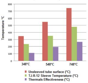
Note: Thermal effectiveness is the difference between the unsleeved and sleeved tube surface temperatures
